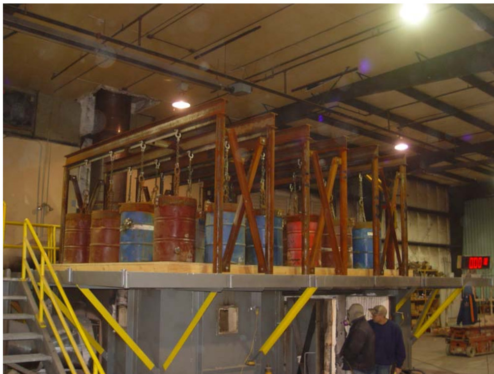
Figure 3: Barrels Mounted on Test Assembly
