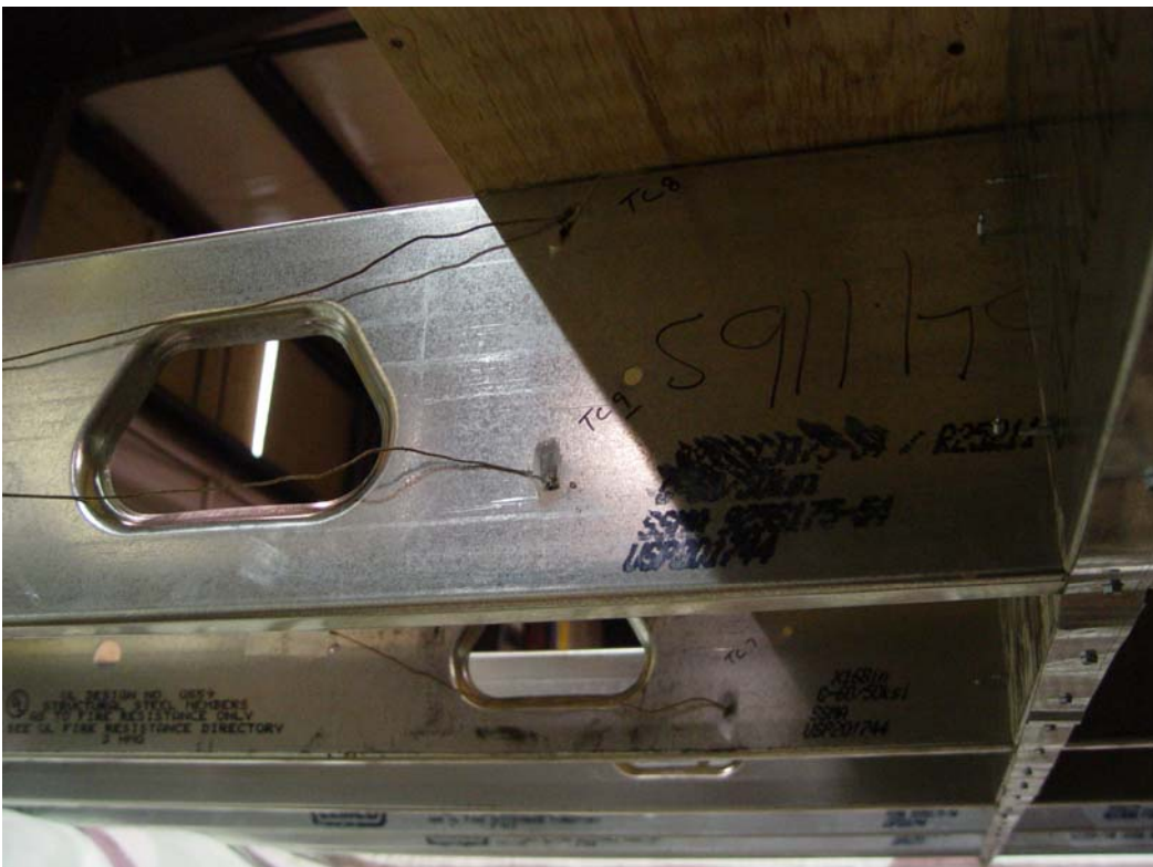
Location of Cavity Thermocouples
